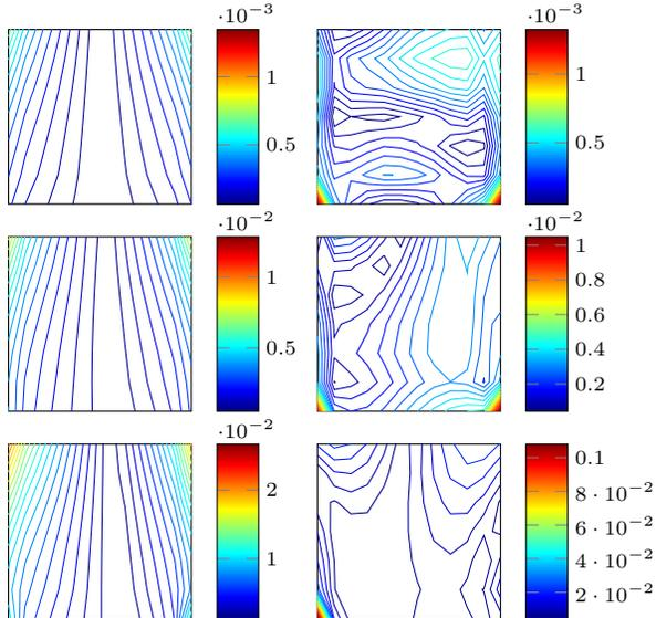
Fig. 6. The relative errors between the stream function contours generated from the bilinearized system (left) and reduced-order system (right) at  $t = 0.01s, 0.05s$  and steady state, respectively (from top to bottom).
