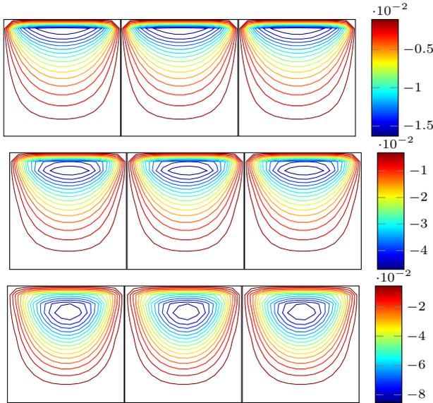
Fig. 5. Stream function contour generated with full-order system (left side), bilinearized system (middle) and reduced-order system (right side) at  $t = 0.01s, 0.05s$  and steady state, respectively (from top to bottom).
