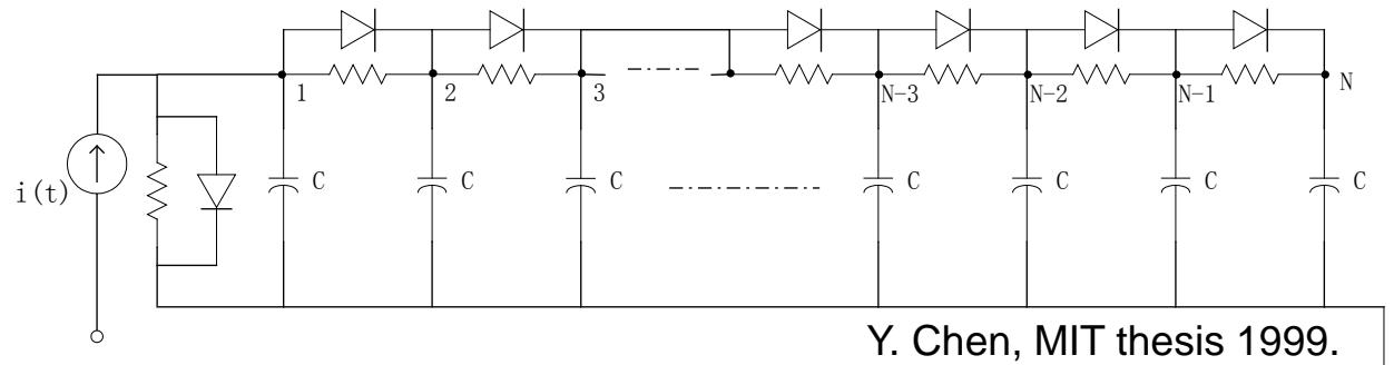
$$\frac{dX}{dt} = \begin{bmatrix} -g(x_1) - g(x_1 - x_2) \\ g(x_1 - x_2) - g(x_2 - x_3) \\ \vdots \\ g(x_{k-1} - x_k) - g(x_k - x_{k+1}) \\ g(x_{n-1} - x_n) \end{bmatrix} + \begin{bmatrix} 1 \\ 0 \\ \vdots \\ 0 \end{bmatrix} u(t),$$
