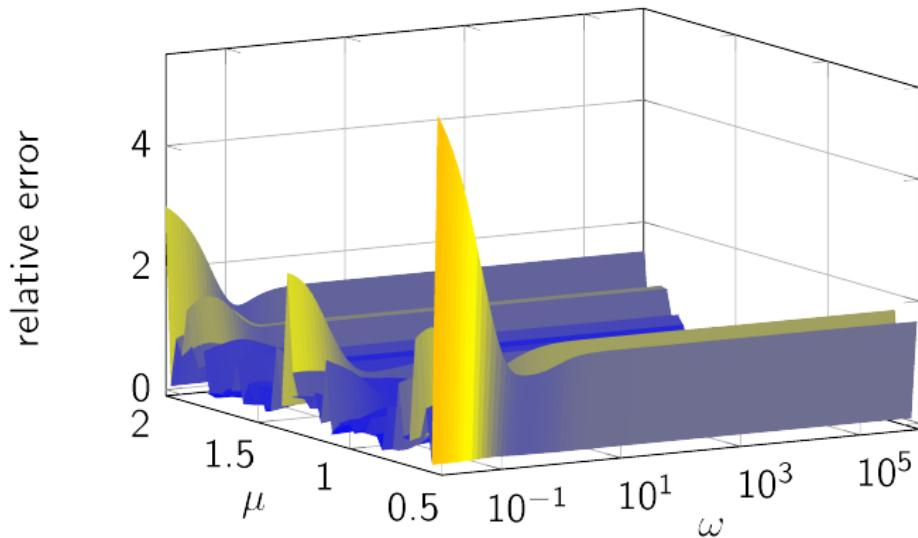
relative error  $\|G(j\omega, \mu) - \hat{G}(j\omega, \mu)\|$  for  $k = 5$  interpolation points.
