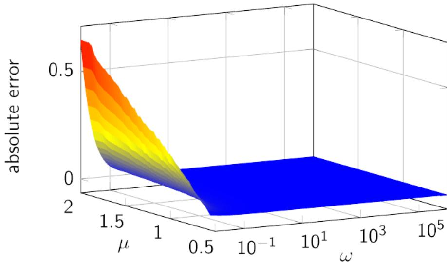
absolute error  $\|G(j\omega, \mu) - \hat{G}(j\omega, \mu)\|$  for  $k = 5$  interpolation points.
